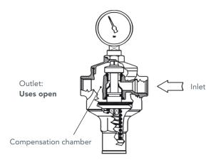
When the uses are opened downstream, the pressure exerted on the piston is lessened in favour of the force exerted by the spring on the shutter permitting it to open with the constant passage of the fluid. As the water demand from the user network increases the pressure on the piston decreases and more water passes.
