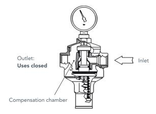
When the uses to be served are closed, the downstream pressure increases, pushing the reducer piston downwards. In this way, the shutter closes the passage section of the reducer maintaining the setting value set on the spring constant; in fact, the minimum pressure difference across the shutter permits the perfect closing of this latter.
