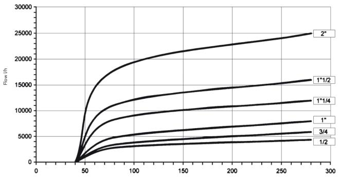
Pressure loss kPa (1 kPa = 101 mm  $H_2$ 0)
