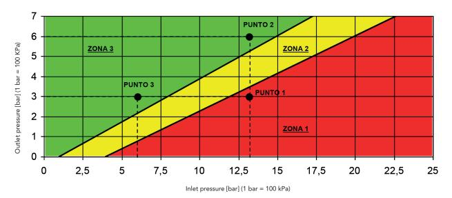
In order to avoid cavitation phenomena and therefore excessive component noise, we recommend choosing the number of pressure reducing valves necessary for a determinate pressure differential, according to the information in the "CAVITATION DIAGRAM".
